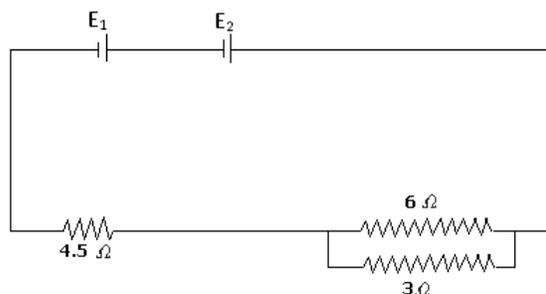
Calculate the value of current flowing through the resistance of  $3\Omega$ .
