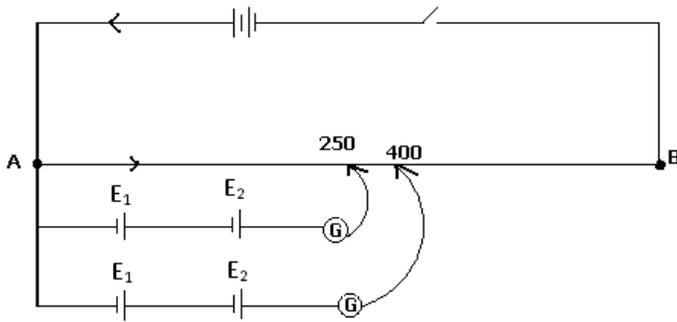
If the balancing lengths for the two combinations of the cells are 250 cm and 400 cm, find the ratio of  $E_1$  and  $E_2$ .
